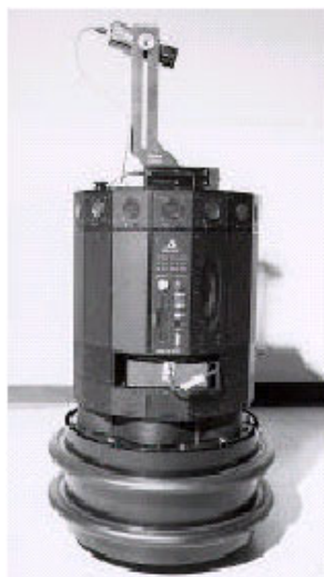
Figure 6. The Nomad 200 is a mobile robot equipped with a ring of 16 sonar sensors.
